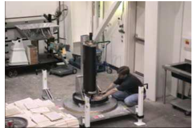
Qual boom ready for thermal balance test
